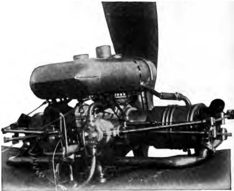
Fig. 19. Clement Two-Cylinder Water-Cooled Motor
